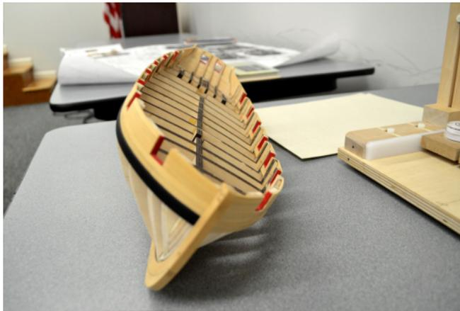
A unique feature of these vessels was the planking at the stern, a design called the square tuck (as opposed to the rounded design common in ships like *Warrior*). This rabbeted design was utilized to cover the end grain of the planks, thereby exposing less area to potential rot. It was also common on fir-constructed ships, vessels built with the softer wood that were not expected to last a long time.
