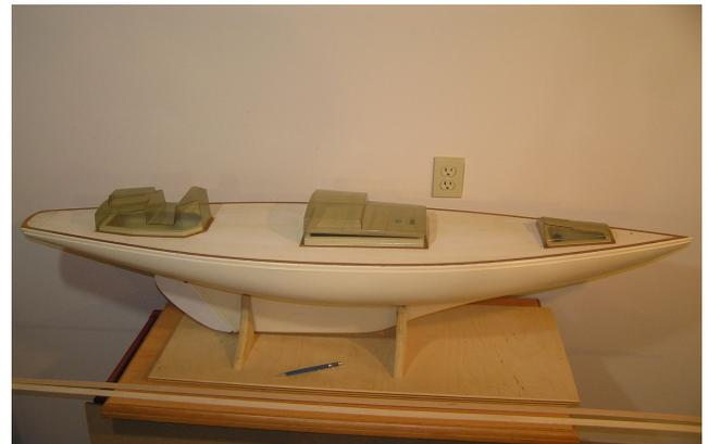
The bulwarks were •screwed in at strategic points and countersunk. DAP Insta Cure Adhesive was progressively applied. The bow ‘fit’ was achieved using card scraper w/sand paper on two sides. A doll house molding, hand applied, simulating lower molding treatment of original bulwarks. The molding hid the void at intersection of hull rabbet and bulwark.
