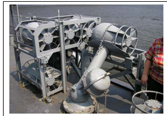
Starboard side K-Gun and Depth Charge Rack with Mk 9 Tear Drop Charge
