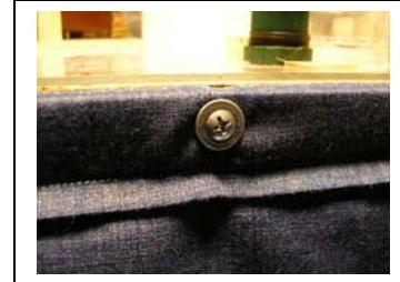
I also found that the product needs to be supported at both ends; otherwise, the small brass screws begin to pull out of the pine components as shown below.
