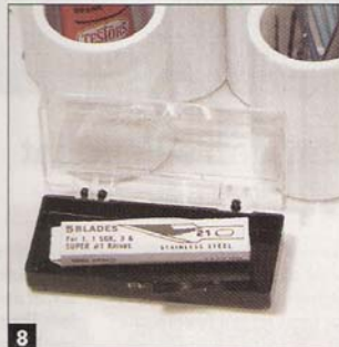
8 A small, snap-lid box glued to the base provides storage for spare hobby-knife blades.
