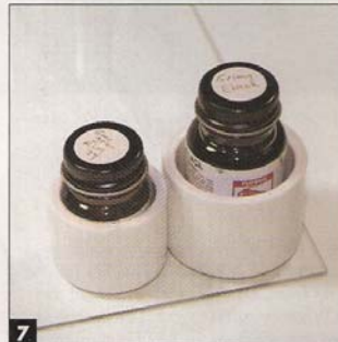
7 End caps at the front edge of the caddy are a great way to prevent knocking over expensive paint bottles.
