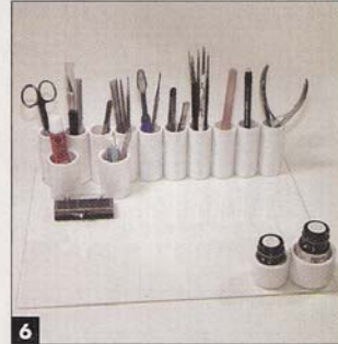
6 After about 30 minutes, I loaded up the caddy with tools. A piece of rubber or cork in the bottom of each tube protects the tool points.
