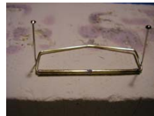
Photo 5 – The basic frame has been inserted into the tubing and is ready to be soldered.
