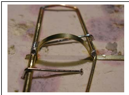
Photo 6 – The center bar has been positioned and is ready for soldering. Note the small pieces of Stay Brite solder positioned on the piece.
