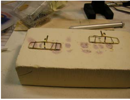
Photo 8 – Two frame assemblies have been pinned to a magnesium block for soldering.
