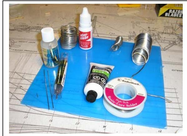
Clockwise from the lower left corner is TIX solder and flux (melts at  $< 300^{\circ}\text{F}$ ), a Stay Brite Silver Solder kit (includes the solder and flux), coils of lead free solid core solder that came with soldering irons and a tube of flux that came with the Bernz-O-Matic torch and a coil of rosin core solder from Radio Shack.
