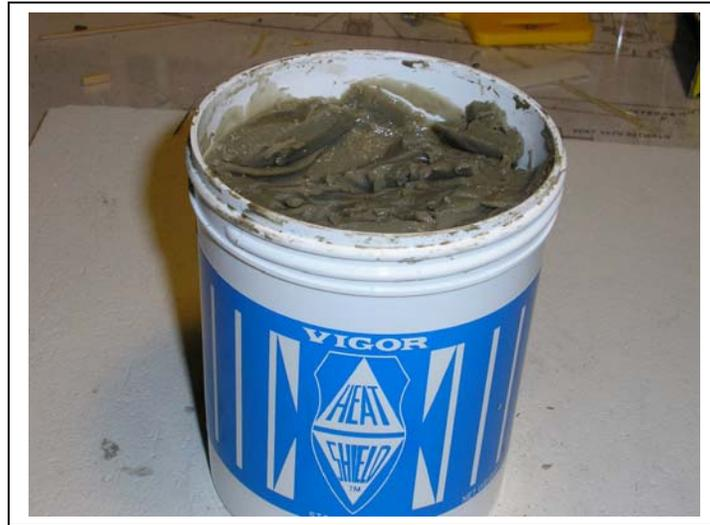
A 16oz container of Heat Shield is above. It is easy to apply and protects soldered joints from heat being applied to new solder areas. It cleans up with easily with water.
