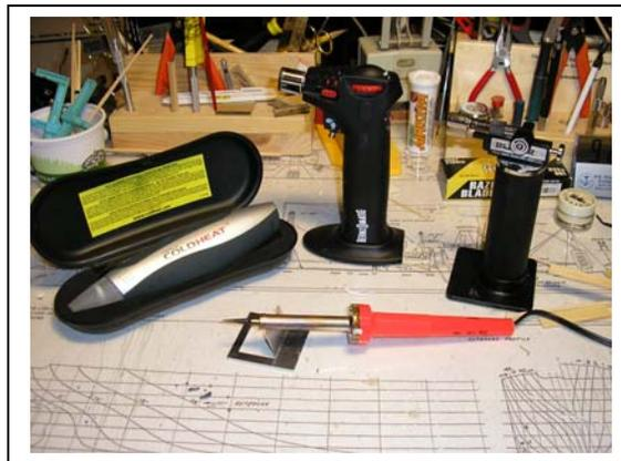
From left to right are a Cold Heat Soldering Gun, a Bernz-O-Matic Butane Torch, a Blazer Micro Torch and a 40 watt soldering iron.
