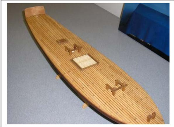
**Tony Alworth's** latest project is the Model Shipways kit of the *Willie F. Bennett*, a Chesapeake Bay skipjack built in 1890. The scale is  $3/8" = 1'$ . The model is built like a real skipjack, on molds. Tony chose to have an open interior and has added the deck beams and carlins. Of about 1,000 skipjacks built, only 30 still exist.
