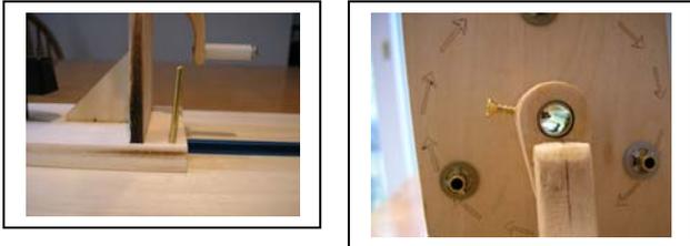
I happened to have #2 – 1/2" brass screws on hand so that is what I used, drilling a pilot hole into the handle and axel.
