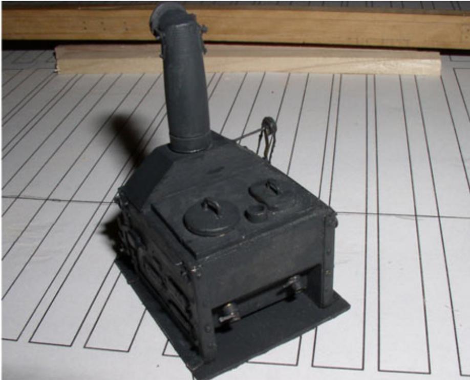
Photo 13 shows the drain valves. I made these on the lathe. The drain pipe then had a small hole drilled in the side to take the valve handles which are no more than small pieces of brass rod that were pounded flat on one end.
