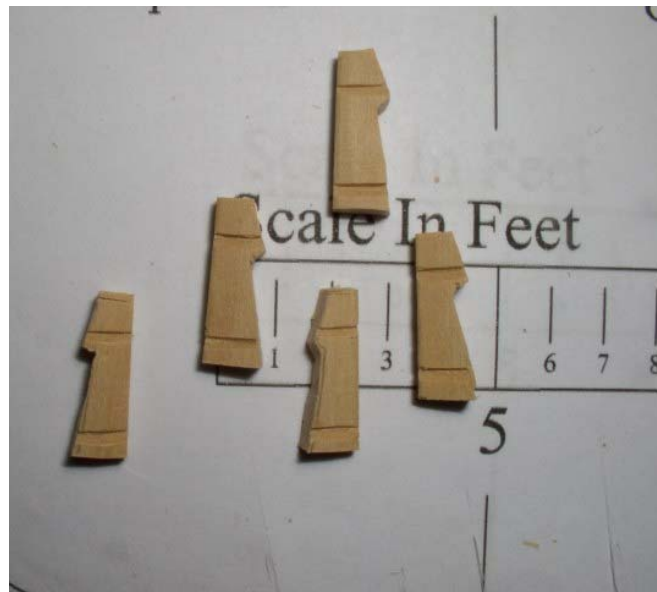
Lower capstan rough cut whelps with grooves for chocks
