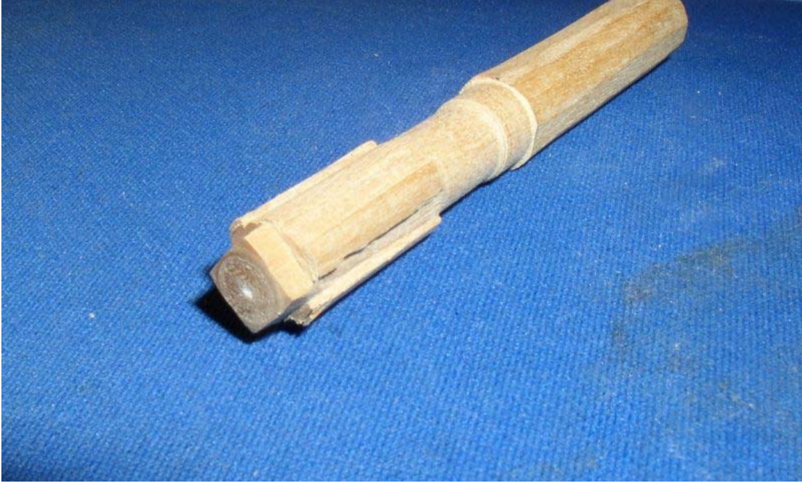
Barrel showing squared top and bottom portion not yet grooved for whelps
