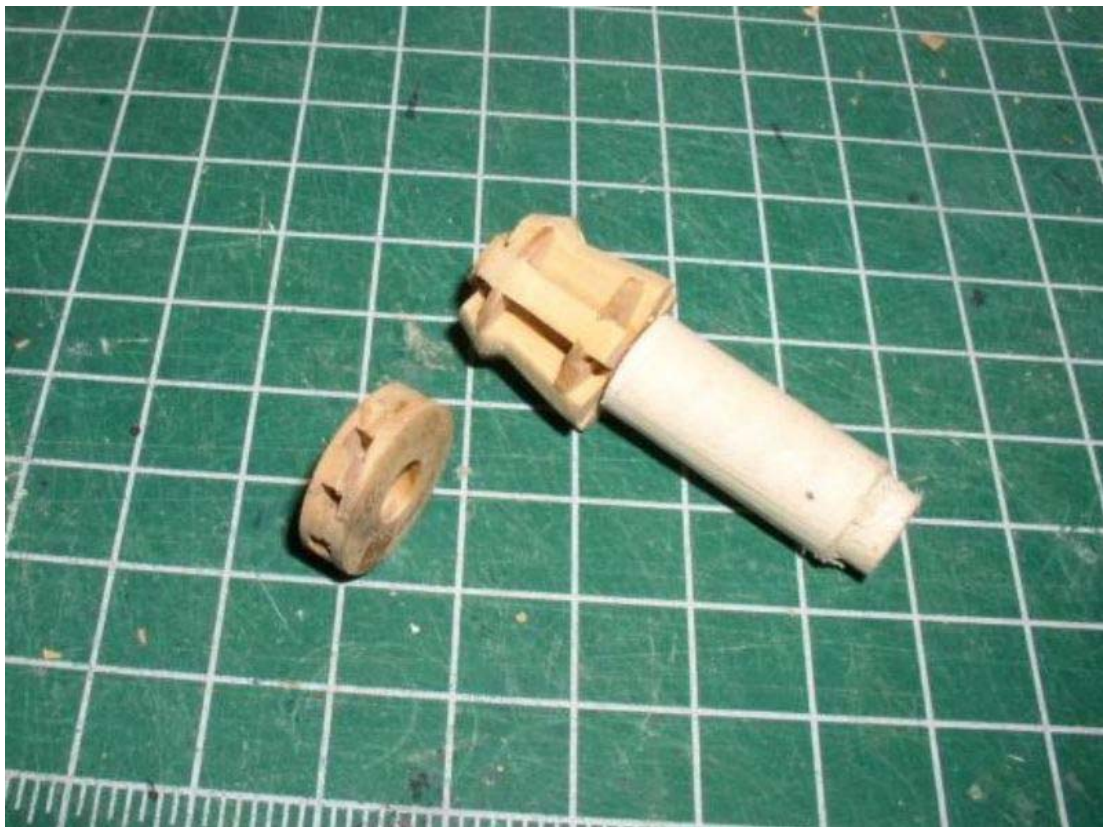
Upper capstan head and body with temporary dowel
