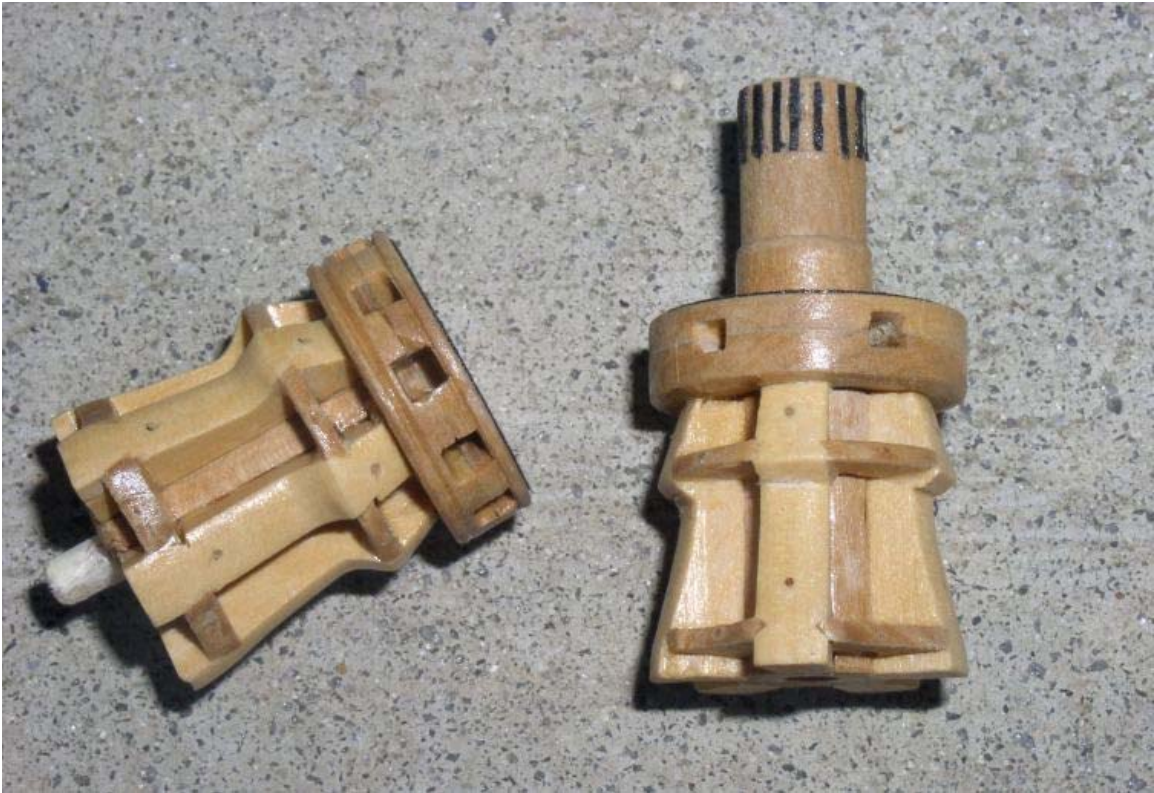
Finished lower and upper capstans
