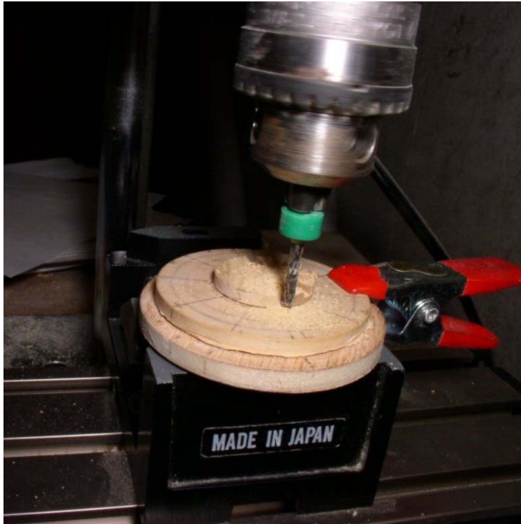
The moveable disk is clamped in place while a groove is cut.
