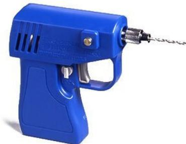
Larry Friedlander provided more details about the [Tamiya battery operated hand drill kit](#) he had introduced at the December meeting. Assembly was easy and it works well for light duty drilling. No gluing is involved. Tweezers are handy and only a screw driver is needed. The drill is relatively high torque and low RPM so it won't melt plastic. The collet will handle a size 6 or 7 drill bit. Per Larry: "It's fun! It's cute! Nice gift for a kid".
