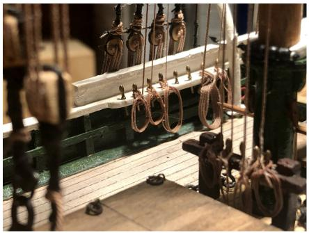
Peter's method made narrower coils which came in handy on my fore pin rails where there were many coils tightly packed.
