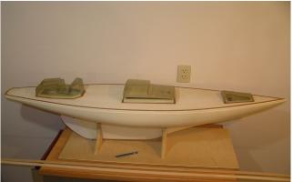
The bulwarks were •screwed in at strategic points and countersunk. DAP Insta Cure Adhesive was progressively applied. The bow 'fit' was achieved using card scraper w/sand paper on two sides. A doll house molding, hand applied, simulating lower molding treatment of original bulwarks. The molding hid the void at intersection of hull rabbet and bulwark.
