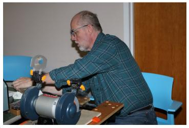
start with a chisel that is already the correct geometry, you would normally only need to grind it if you are repairing damage.
