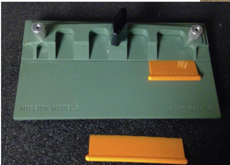
As part of his photoetch demonstration, Tom demonstrated a bending jig for photoetch. The unit is hard plastic and has several shapes of various sizes. There are four different size wedges. The part to be bent is clamped under one of the fingers and then a wedge is used to lift the portion to be bent. It is from Mission Models.
