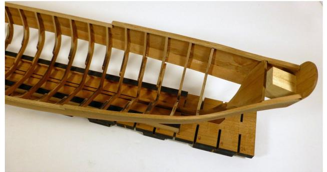
This model is Winchelsea that Joe has restarted after a long drawn out completion of a model a group of us did for a local privately owned museum. Joe thickness sanded and milled some left over Alaskan Yellow Cedar sheet stock from for the underlay-ment of the wales. The clamps near the bow are holding shim stock glued to the inside of the wales to flatten the slight "bulges" to minimize sanding.
