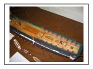
**HENRY SCHAEFER** showed us his completed model in large scale of the tug *Ocean Prince*. This is the fourth copy of the vessel that Henry has built. The previous versions having been given to others, Henry wanted one for himself. The model is plank on bulkhead and uses parts from various suppliers although Henry scratch built many of the hardware and fittings. On larger models like this Henry uses Krylon spray paints which he considers first rate.
