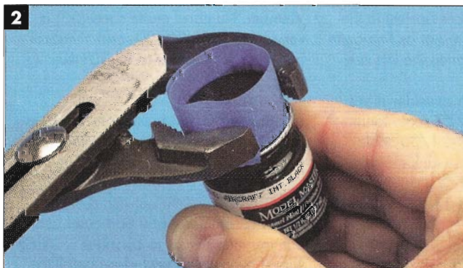
2 Slip-joint plumber's pliers will give you plenty of extra leverage, but be careful not to bend the cap or break the bottle!
