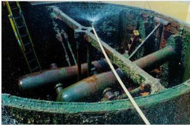
USS Monitor's XI-inch Dahlgren Shell Guns upside down inside the turret prior to conservation, Mariners' Museum in Newport News, Virginia (Photo by Jim Janke, August 2004).
