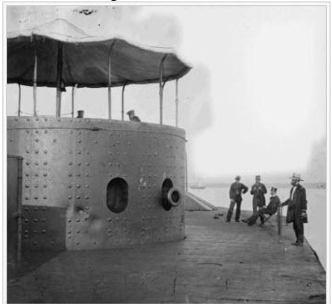
On the Deck of the USS Monitor , a XI-inch Dahlgren Shell Gun peeking out it's porthole. Hampton Roads, Virginia. (Library of Congress Photo, July 9, 1862).
