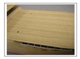
The decking is fabricated using the method Bob illustrated in a previous tech session which utilizes several layers of veneer laminated into a block and then ripped into thin sections. Once the sections are butted together, the effect is a deck of individually laid planks.
