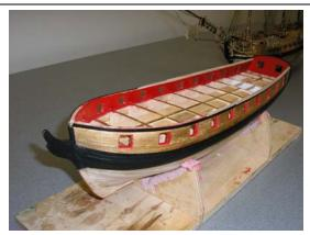
**Ray Vernon** brought in his model of HMS *Surprise*, originally built by the French in 1974 and captured by the British in 1796 and renamed *Surprise*. The kit is plank on bulkhead in 1:75 scale. The vessel was the subject of Patrick O'Brian's novels.
