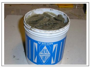
A 16oz container of Heat Shield is above. It is easy to apply and protects soldered joints from heat being applied to new solder areas. It cleans up with easily with water.
