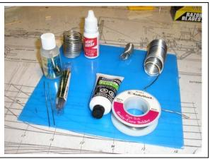
Clockwise from the lower left corner is TIX solder and flux (melts at < 300°F), a Stay Brite Silver Solder kit (includes the solder and flux), coils of lead free solid core solder that came with soldering irons and a tube of flux that came with the Bernz-O-Matic torch and a coil of rosin core solder from Radio Shack.
