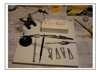
Some useful accessories are to the left. The tools are on a 12"x12" soldering board. A magnesium block is at the top. The items at the bottom right are aluminum heat sinks and to their left are a couple of soldering picks.
