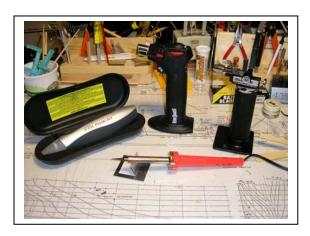
From left to right are a Cold Heat Soldering Gun, a Bernz-O-Matic Butane Torch, a Blazer Micro Torch and a 40 watt soldering iron.
