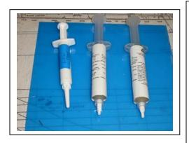
Above are silver solder pastes in soft, medium and hard grades. The paste is a mixture of silver solder and flux.
