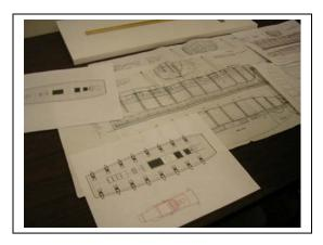
The last model Dan discussed is another kit model he is building for a client, the racing yacht *America* built in 1851. It is a Bluejacket kit in 1:48 scale of plank on frame construction. The hull frames are of Basswood. Dan explained Bluejacket's method of creating the individual frames included in the kit which are sawn from a solid hull form, just like cutting a loaf of bread.
