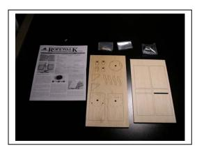
All parts were easily removed from the sheets by hand. I did not need to use cutting tools at all. I did have a problem with the geared end upright piece, however. The laser did not cut through the wood entirely on one of the gear axel holes.
