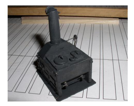
Photo 13 shows the drain valves. I made these on the lathe. The drain pipe then had a small hole drilled in the side to take the valve handles which are no more than small pieces of brass rod that were pounded flat on one end.
