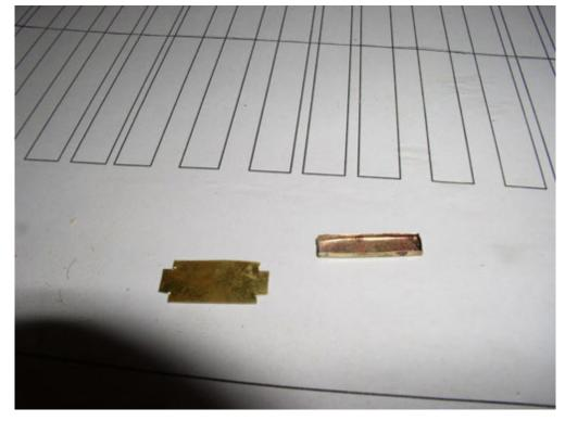
Photo 17 shows the drip pan that sits at the base of the grill area. Mine is made of 0.050 brass sheet as mentioned above. The photo shows a piece that is not yet bent, and second shows it bent and silver soldered. It looks a little beat, but I am sure that was the case on board the real ship.
