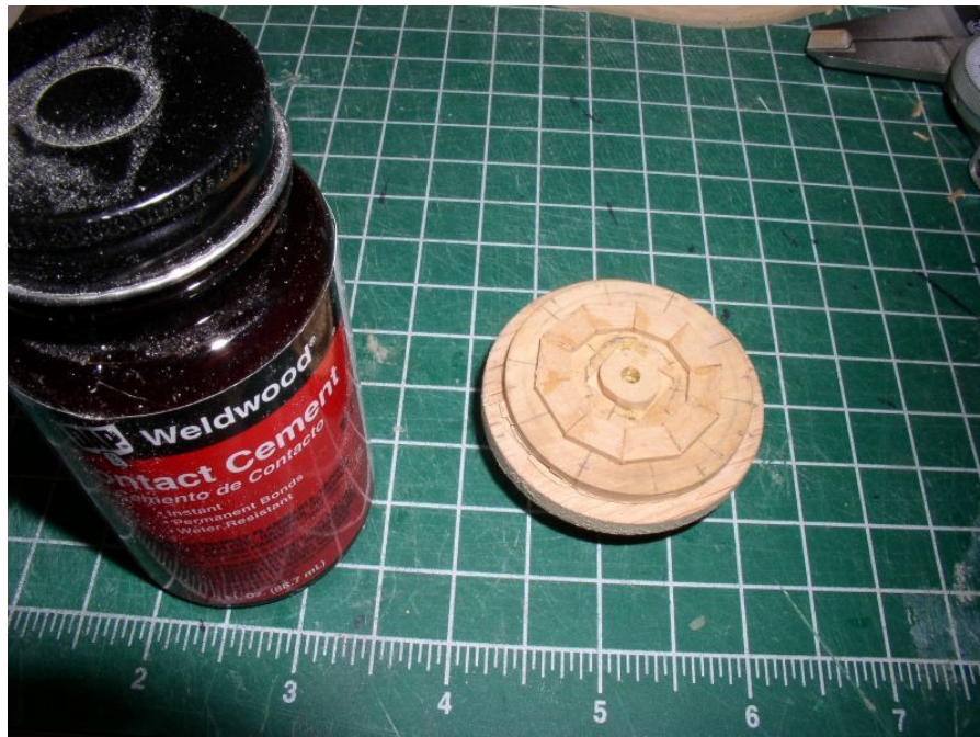
Hub and Rim temporarily cemented on the Lazy Susan
