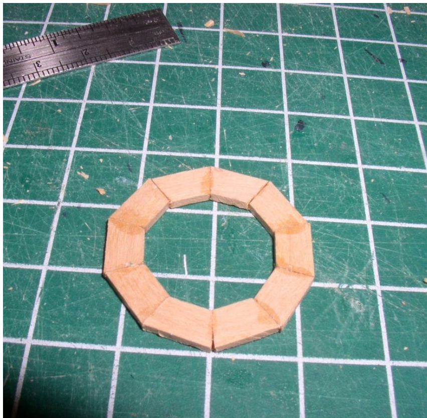
Rim segments epoxy glued together – note the slight gap. This will be gone as it is outside the finished OD of the wheel
