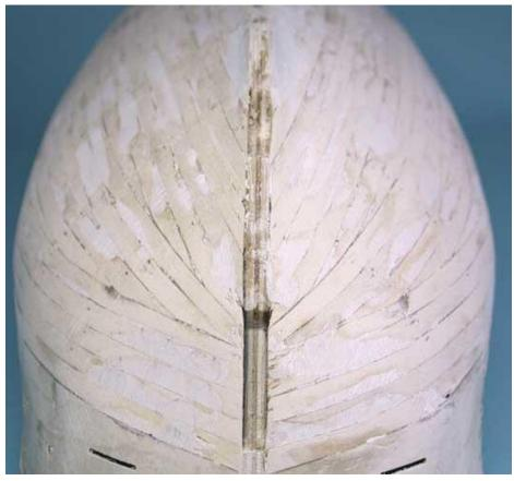
Planking with no stealers or drop planks below the wales. Avoid This!!
